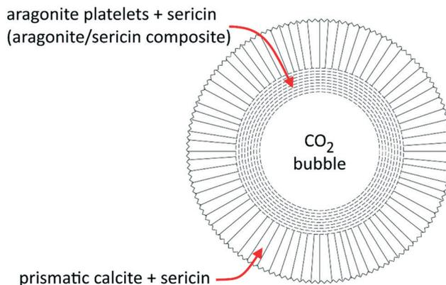
Fig. 5 Structure of the spherulite grown in the presence of sericin. Around the core cavity (a  $\text{CO}_2$  bubble) aragonite and calcite grow in concentric shells. Modified from Pastero and Aquilano.<sup>34</sup>
