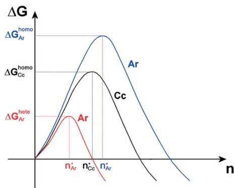
**Fig. 6** Qualitative activation energies ( $\Delta G_{Ar}^{hete}$  and  $\Delta G_{Ar}^{homo}$ ) and critical nuclei ( $n_{Ar}^*$ ) for heterogeneous (red line) and homogeneous (blue line) nucleation of aragonite, Ar, in supersaturated aqueous solutions. The activation energy and critical nucleus for homogeneous nucleation (black line) of calcite, Cc, are also reported ( $\Delta G_{Cc}^{homo}$  and  $n_{Cc}^*$ ).
