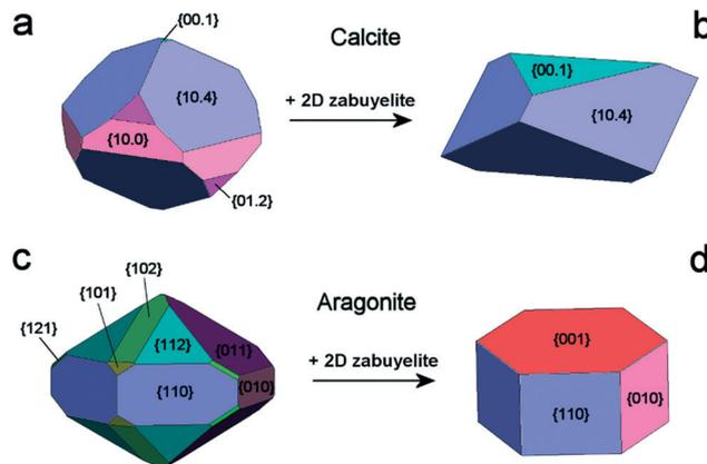
Fig. 3 Equilibrium shapes of calcite and aragonite at 0 K. Calcite (a) and aragonite (c) in the vacuum; calcite (b) and aragonite (d), after the 2D-epitaxial adsorption of zabuyelite above  $(00.1)_{\text{Cc}}$ ,  $(10.4)_{\text{Cc}}$  and  $(001)_{\text{Ar}}$ . Redrawn from Aquilano *et al.*<sup>46</sup>
