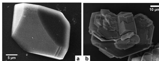
**Fig. 2** Calcium carbonate polymorph grown in the presence of lithium in solution: (a) calcite cleavage rhombohedron with initial rounding of corners and apices (modified from Aquilano *et al.*<sup>46</sup>); (b) prismatic aragonite crystals associated with flat, pseudo-hexagonal calcite crystals (modified from Aquilano *et al.*<sup>16</sup>).
