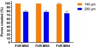
**Fig. 4** Insertion test in the Parafilm® skin simulant model: Percentage of MNs that penetrated the first two Parafilm® layers (140  $\mu$ m and 280  $\mu$ m depth, respectively) by FUR-MNs, results expressed as means  $\pm$  s.d., n=3.
