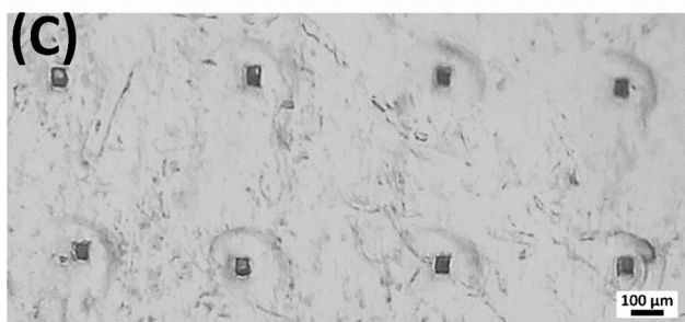
Fig. 5 Insertion test in the Parafilm® skin simulant model. (A) The side length of the pores created by MNs on the first two Parafilm® layers ( n = 10 , mean ± s.d.). Representative microscopic images of Parafilm® into which FUR-MN2 was inserted: (B) first layer (140 μm), (C) second layer (280 μm). Scale bar 100 μm.
