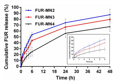
Fig. 10 In vitro drug release from microneedles containing varying concentrations of FUR (pH 7.4, 37  $^{\circ}$ C). Inset shows the drug release profile over the initial 6 h. Values are mean  $\pm$  s.d. of four experiments.
