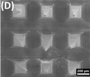
Fig. 3 Representative SEM images of the obtained microneedles: (A) P-MN, (B) FUR-MN2, (C) FUR-MN3, and (D) FUR-MN4. Scale bar 200 µm.
