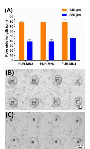
Fig. 5 Insertion test in the Parafilm® skin simulant model. (A) The side length of the pores created by MNs on the first two Parafilm® layers (n=10, mean  $\pm$  s.d.). Representative microscopic images of Parafilm® into which FUR-MN2 was inserted: (B) first layer (140  $\mu$ m), (C) second layer (280  $\mu$ m). Scale bar 100  $\mu$ m.
