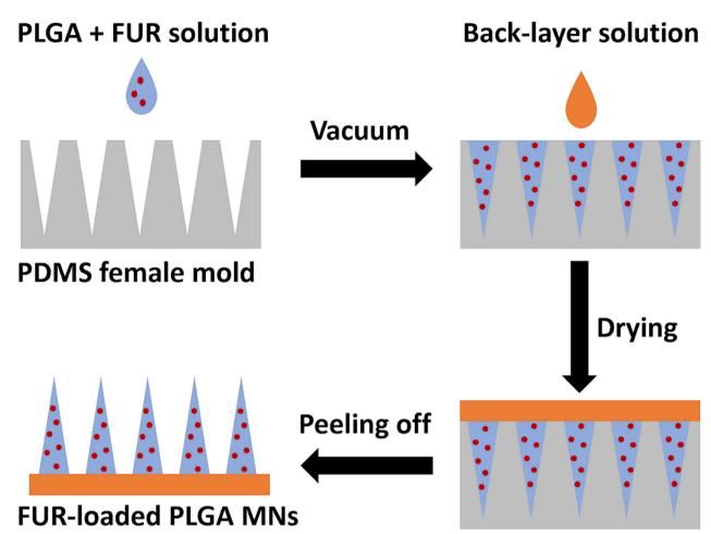
Fig. 1 Preparation scheme of FUR-loaded PLGA MNs using a polydimethylsiloxane (PDMS) microneedle mold.
