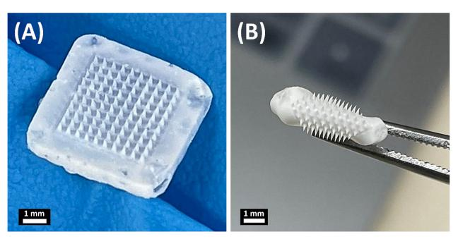
Fig. 2 Representative images of the obtained microneedles: (A) FUR-MN2 and (B) folded FUR-MN2. Scale bar 1 mm.
