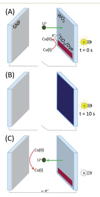
Fig. 2 Schematic diagram of the PECD in: (A and B) open-circuit conditions under simulated sunlight (at t=0 and after 10 s); (C) short-circuit under dark conditions. The oxidation and reduction of the Y123 dye is not drawn so as not to complicate the readability of panels (A) and (C).
