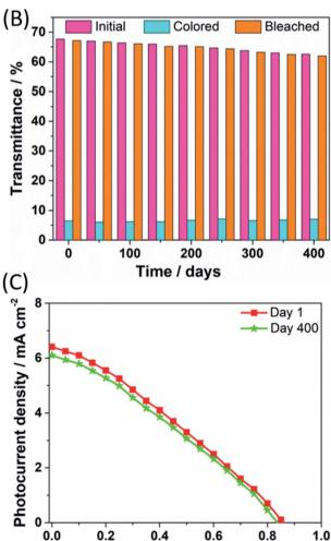
Fig. 4 (A) PhCE of the PECD under 1 sun irradiation, comparing the values calculated at day 1, day 200 and day 400 of the ageing test. The inset shows pictures taken at day 400 under colored and bleached conditions, respectively. (B) Luminous transmittance vs. ageing time for the PECD. (C) J-V curves of the DSSC portion of the PECD, measured under 1 sun irradiation (AM 1.5G) just after fabrication and at day 400 of the ageing test
