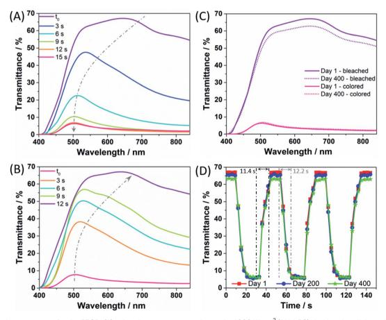
Fig. 3 Transmittance spectra for the PECD: (A) coloration process occurring under 1000 W m<sup>-2</sup> (AM 1.5G) simulated sunlight and (B) bleaching process taking place under short-circuit and dark conditions. (C) Transmittance modulation of the PECD under bleached and colored conditions, comparing the spectra at day 1 and day 400 of the ageing test. (D) Transient transmittance response time for the PECD, comparing the traces at day 1, day 200 and day 400 of the ageing test.
