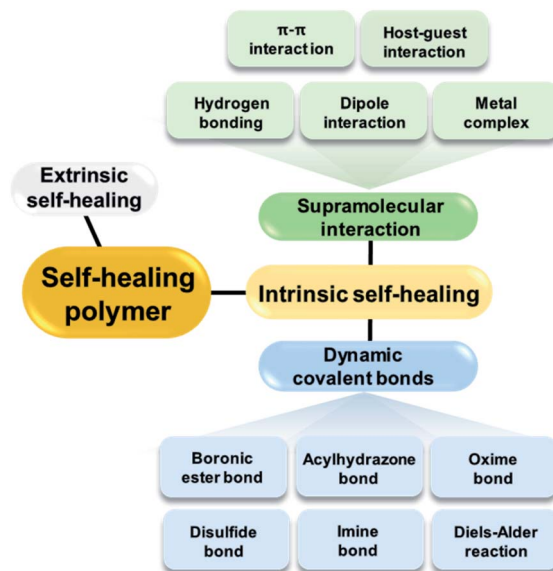
Fig. 1 Strategies used to prepare self-healing polymers.
