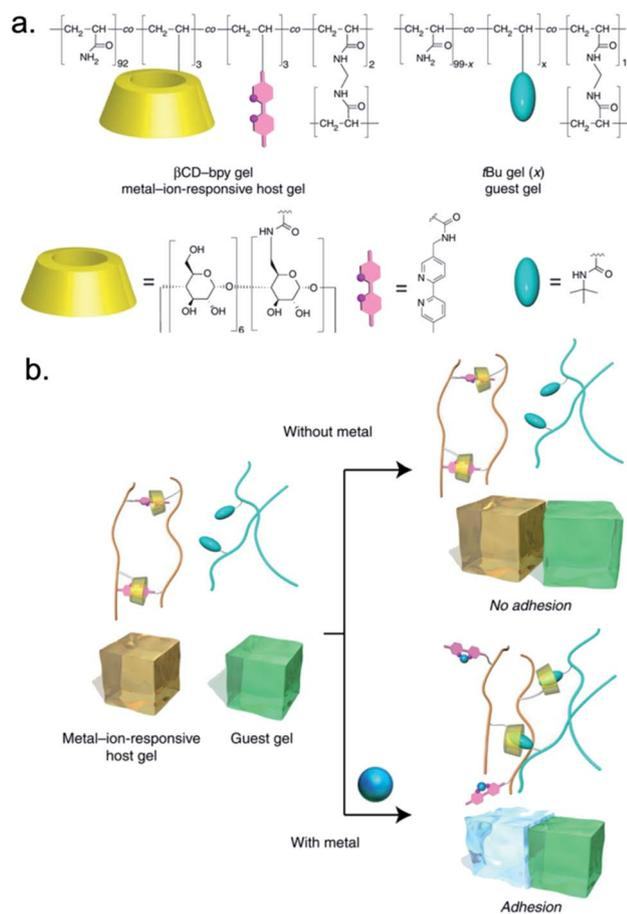
Fig. 10 Metal-ion mediated interfacial adhesion based on host-guest interactions between two hydrogels. (a) Structures of  $\beta$ CD-BIPY hydrogel and *N*-tBuAAm hydrogel. (b) Metal ion modulates adhesion by forming new host-guest interaction between  $\beta$ CD-BIPY hydrogel and *N*-tBuAAm hydrogel. Adapted from ref. 68. Copyright 2014 Springer Nature (<http://creativecommons.org/licenses/by/4.0/>).<sup>68</sup>
