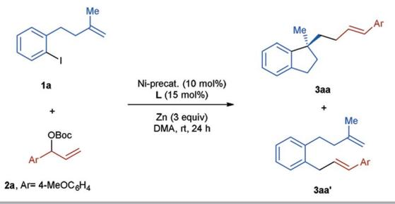
Reaction scheme showing the optimization of the reaction conditions. Substrate **1a** (an aryl iodide-tethered alkene) reacts with allylic carbonate **2a** (Ar = 4-MeOC<sub>6</sub>H<sub>4</sub>) in the presence of a Ni-precatalyst (10 mol%), ligand **L** (15 mol%), Zn (3 equiv), and DMA at room temperature for 24 hours to yield products **3aa** and **3aa'**.
