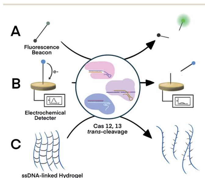
Fig. 2 Three representative nucleic acid detection platforms using the *trans*-cleavage activity of CRISPR–Cas12a and –Cas13a. *Trans*-cleavage of ssDNA or ssRNA linker built into (A) a fluorophore and quencher pair,<sup>50,51</sup> (B) a redox-reactive molecule and electrode,<sup>53,54</sup> or (C) hydrogel.<sup>55</sup> Adapted from ref. 50 and 54. Copyright 2017 Wiley and Sons.
