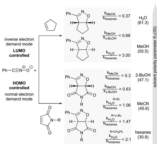
Fig. 19 Influence of solvent polarity on reaction rate.<sup>74</sup>
