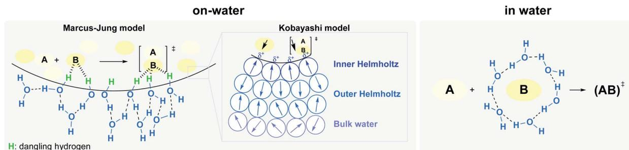
Fig. 5 Hydrogen bonding under heterogeneous (left) and homogeneous (right) conditions, at the oil–water interface, and Kobayashi's partial polarization approach (center).
