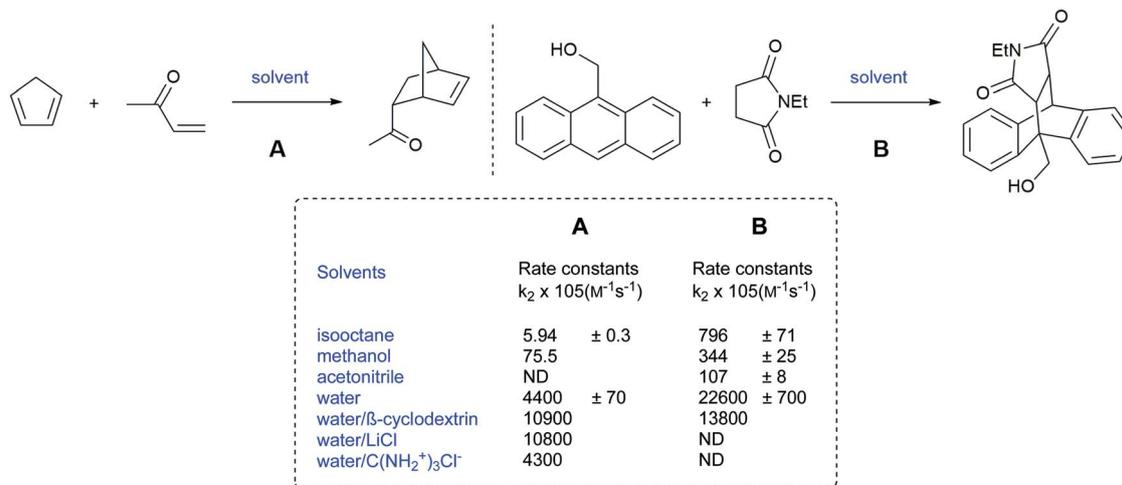
Fig. 2 Diels–Alder reactions accelerated by “on water” conditions (Breslow).<sup>5</sup>
