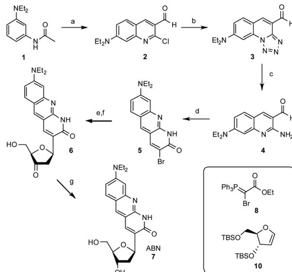
Fig. 2 Synthesis of the ABN nucleoside analogue. Reagents, conditions, and yields: (a) DMF,  $POCl_3$ , 50 °C, 20 min (15%). (b)  $NaN_3$ , DMF, 90 °C, 18 h (85%). (c)  $PPh_3$ , 2 N HCl, reflux, 2 h (70%). (d) **8**, NaOEt, ethanol, 70 °C, 4 h. (e) **10**,  $AsPh_3$ ,  $Pd(OAc)_2$ ,  $Bu_3N$ , 60 °C, 18 h. (f) TBAF, AcOH, rt, 1 h. (g)  $NaBH(OAc)_3$ , AcOH,  $CH_3CN$ , 0 °C, 1 h (9% over 4 steps).
