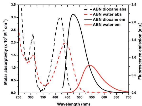
Fig. 4 Absorption (dashed line) and emission (solid line) spectra of ABN in dioxane (black) and water (red). The integral areas of emission spectra are normalized to brightness  $\epsilon \cdot \Phi_{\text{em}}$ .
