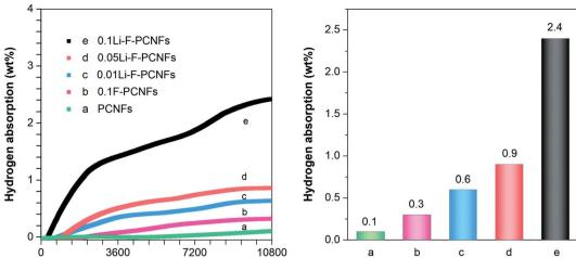
Fig. 7 Hydrogen adsorption spectra (left) and capacities (right) of (a) PCNFs, (b) 0.1 F-PCNFs, (c) Li-0.01F-PCNFs, (d) Li-0.05F-PCNFs, and (e) Li-0.1F-PCNFs composites at 0 °C under a hydrogen pressure of 10 MPa.
