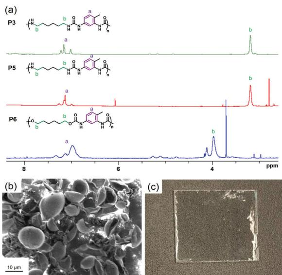
**Fig. 3** (a) <sup>1</sup>H-NMR spectra of polyurea/urethane nanocapsules (entries P3, 5 and 6) in acetone-*d*<sub>6</sub>:TFA (40:60). (b) SEM micrograph of polyurea microcapsules prepared by interfacial polymerization in an oil-in-water emulsion. (c) Photograph of a polyurethane coating prepared by the reaction between resorcinol and HMDI.
