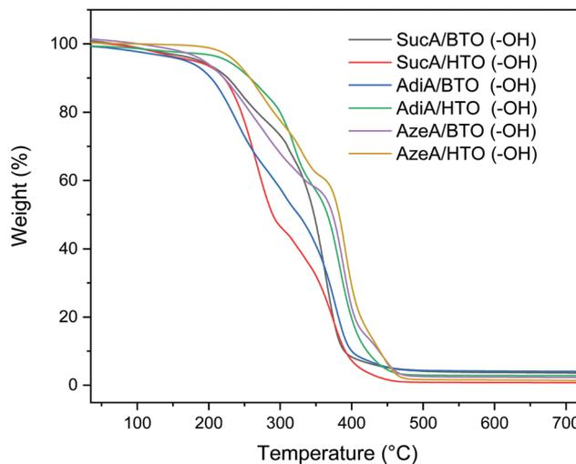
Fig. 5 TGA thermograms of hydroxyl-terminated branched polyesters.
