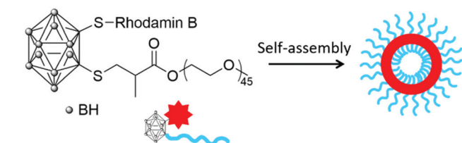
Scheme 2 Self-assembly into vesicles of a fluorescent carborane-conjugated POEGMA.
