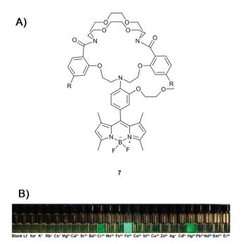
Fig. 4 (A) Cryptand-bodipy based sensor 7 for the detection of Fe<sup>3+</sup>. (B) Naked-eye fluorescence responses of 7 (7 µM) in H<sub>2</sub>O-CH<sub>3</sub>CN (9:1) upon addition of 100 equiv. of various metal cations ( $\lambda_{ex}$  = 365 nm). Reproduced with permission from ref. 29, copyright American Chemical Society.
