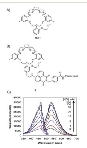
Fig. 1 (A) Ttriazacryptand[2,2,3]-1-(2-methoxyethoxy) benzene (TAC). (B) He's design for an optical sensor. (C) Excitation and emission spectra of a sensor disk exposed to different potassium chloride solutions in TRIS-HEPES buffer at pH 7.40 (left, excitation spectra, fixed emission at 540 nm; right, emission spectra, fixed excitation at 470 nm. Reproduced with permission ref. 32, copyright American Chemical Society.
