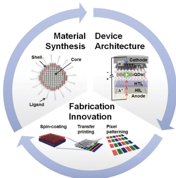
**Fig. 1** Classification of the development categories for QD-LEDs. Performances of QD-LEDs can be elevated by the combination of technology for QD material synthesis, device optimisation and fabrication process.
