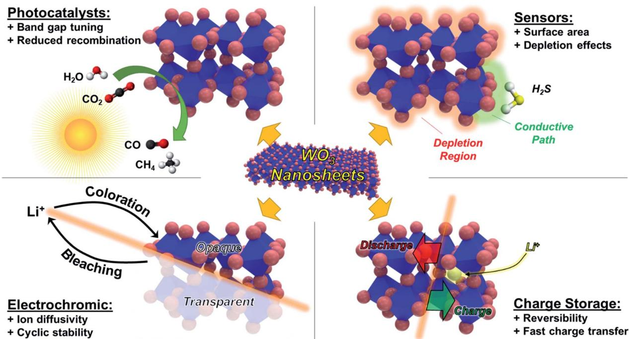
Fig. 1 Schematic showing basic principles of operation for  $\text{WO}_3$  in photocatalysts, sensors, electrochromic devices, and charge storage applications, along with the potential advantages provided by the nanosheet morphology.
