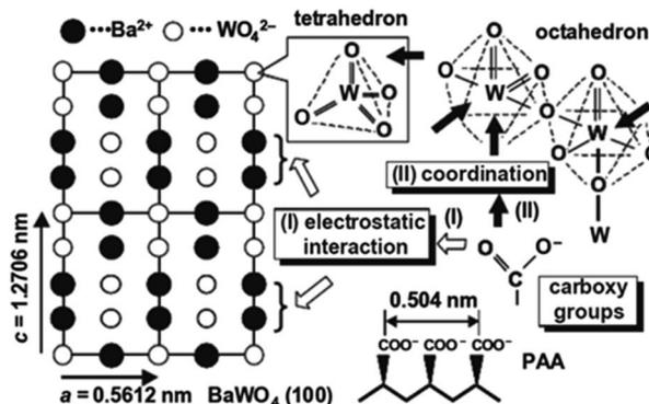
Fig. 4 Illustration of  $\text{BaWO}_4$  (100) and the interaction with PAA molecules that leads to formation of octahedral  $\text{WO}_6$ . Reprinted with permission from ref. 56, copyright 2006, John Wiley and Sons.
