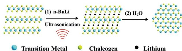
Fig. 8 Intercalation/exfoliation scheme using *n*-BuLi to synthesize TMDC nanosheets. Reprinted with permission from ref. 74, copyright 2016, Royal Society of Chemistry.
