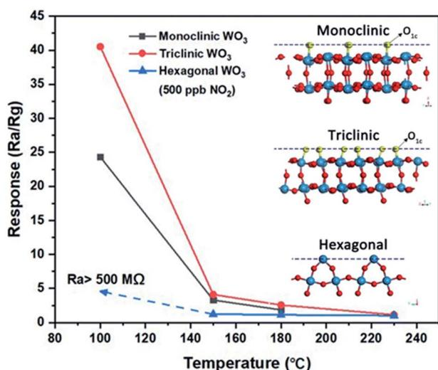
Fig. 12 Effect of WO<sub>3</sub> crystal structure on sensing performance of NO<sub>2</sub>. Inset shows the crystal structures with density of single coordinated oxygen atoms (O<sub>1c</sub>) on the exposed facet. Reprinted with permission from ref. 93, copyright 2020, Springer-Nature.
