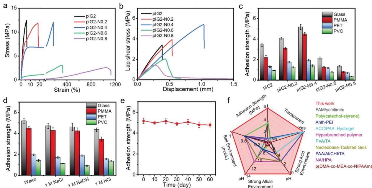
Fig. 3 (a) True stress–strain curves of the pIG2-N samples. (b) Lap shear curves of the pIG2-N samples for glass. (c) Underwater adhesion strength of the pIG2-N samples for different materials. (d) Underwater adhesion strength of pIG2-N0.4 for different materials in different solutions. (e) Long-term stability of the adhesion strength of pIG2-N0.4 in an aquatic environment. (f) Comparison of the underwater adhesion properties of pIG2-N samples and adhesives reported in the literature.
