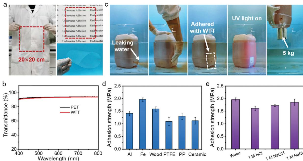
**Fig. 4** (a) Photographs of the waterproof transparent tape with a size of 20 × 20 cm. (b) Transmittance of PET and waterproof transparent tape in the visible wavelength range. (c) Photographs showing the ability of the waterproof transparent tape to repair the hole in a bucket in an aquatic environment. (d) Underwater adhesion strength of the waterproof transparent tape for different materials. (e) Adhesion strength of the waterproof transparent tape with Fe in different environments.
