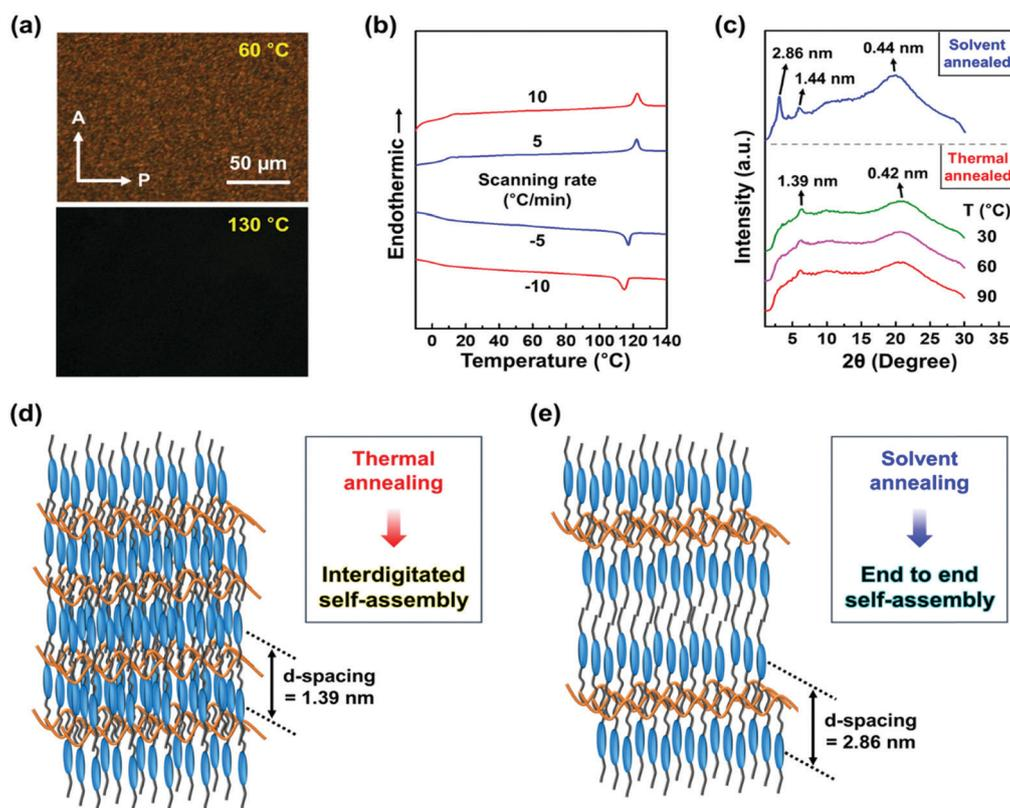
**Fig. 1** Phase transition behaviors of Si-CSM: (a) POM textures at different temperatures, (b) DSC thermograms at different scanning rates, (c) 1D WAXD patterns obtained by different annealing processes, and schematic illustrations of the self-assembled structures obtained by (d) thermal and (e) solvent annealing process.
