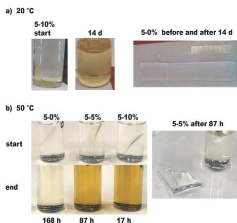
Fig. 6 PU samples before and after degradation test in 5 M HCl in 8 : 2 (v/v) ethanol : H<sub>2</sub>O. (a) Room temperature (b) 50 °C.
