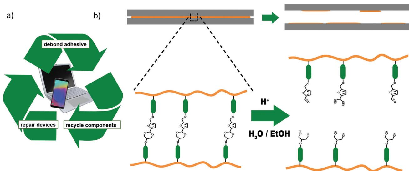
**Fig. 1** (a) Debonding of adhesives can enable the repair of devices by replacing broken parts and the recycling of expensive raw materials. (b) The debonding mechanism proposed in this work: adhesives containing cross-linked PUs with acetal diol additives can be cleaved by acid and aqueous solvent.
