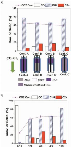
**Fig. 2** Influence of catalyst-bed configuration (a) and catalyst-to-alumina ratio over **Conf. B** (b) on the  $CO_2$  conversion and product distributions in the  $CO_2$  hydrogenation over 15Co catalyst coupled with DBD plasma at the furnace temperature of 250 °C. Reaction conditions: 20 v%  $CO_2$ –60 v%  $H_2$  in Ar balance,  $H_2/CO_2$  = 3, flow rate = 20 mL min<sup>-1</sup>, P=1 atm, voltage = 13.6 kV, frequency = 23.5 kHz, plasma power = 4 W.
