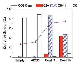
Fig. 3 Influence of catalyst-bed configuration on the CO<sub>2</sub> hydrogenation performance over 15Co catalyst under 10 W of DBD plasma at the furnace temperature of 25 °C. Reaction conditions: 20 v% CO<sub>2</sub>-60 v%  $H_2$  in Ar balance,  $H_2/CO_2 = 3$ , flow rate = 20 mL min<sup>-1</sup>, P = 1 atm, voltage = 18.5 kV, frequency = 23.5 kHz.
