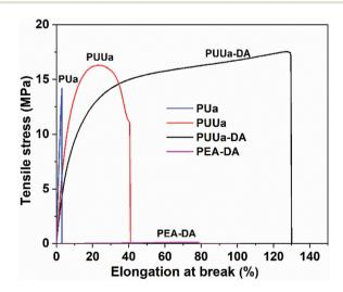
**Fig. 6** Stress–strain curves of polyurea (PUa), polyurethane-urea (PUUa), the polyurethane-urea Diels–Alder adduct (PUUa-DA) and the poly(propylene glycol) bis(2-aminopropyl ether) Diels–Alder adduct (PEA-DA).
