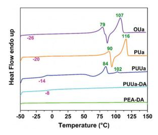
Fig. 5 DSC curves of oligourea (OUa), polyurea (PUa), polyurethaneurea (PUUa), the polyurethane-urea Diels—Alder adduct (PUUa-DA) and the poly(propylene glycol) bis(2-aminopropyl ether) Diels—Alder adduct (PEA-DA) from the second heating scan.
