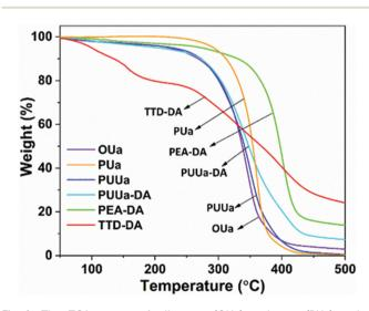
Fig. 4 The TGA curves of oligourea (OUa), polyurea (PUa), polyurethane-urea (PUUa), the polyurethane-urea Diels-Alder adduct (PUUa-DA), the poly(propylene glycol) bis(2-aminopropyl ether) Diels-Alder adduct (PEA-DA) and the 4,7,10-trioxa-1,13-tridecanediamine Diels-Alder adduct (TTD-DA).
