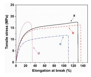
Fig. 9 Stress-strain curves of the polyurethane-urea Diels-Alder adduct (PUUa-DA) before and after cutting and healing at different temperatures and times. (a) Original specimen; (b) healed at 120  $^{\circ}$ C for 10 min and then healed at 60  $^{\circ}$ C for 24 h; (c) healed at 60  $^{\circ}$ C for 24 h; (d) healed at 120  $^{\circ}$ C for 10 min.
