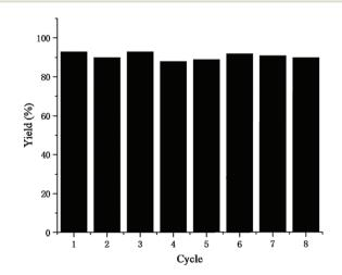
Fig. 3 Recycling experiments using  $AgNO_3$  as the catalyst and [Ch][Triz] as the cocatalyst.
