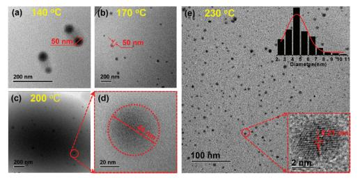
Fig. 1 TEM images of the products obtained at (a) 140, (b) 170, (c) and (d) 200, and (e) 230 °C in ethanol, respectively. The insets are the size distribution histogram (upper right) and the HRTEM (lower right) image of CPDs obtained at 230 °C.
