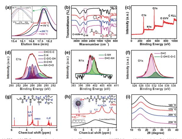
Fig. 2 (a) GPC and (b) FT-IR spectra of products prepared at different temperatures. (c) XPS full scan, (d) high resolution C 1s, (e) high resolution N 1s, and (f) high resolution O 1s of CPDs. (g) <sup>1</sup>H NMR (DMSO-d<sub>6</sub> + D<sub>2</sub>O) spectra of the CPDs. (h) <sup>1</sup>H SSNMR spectra of the CPDs and crosslinked PHUs. (i) WAXS spectra of the CPDs.
