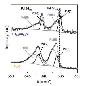
Fig. 3 XPS spectra of Pd 3d in Pd<sub>0.5</sub>Cu<sub>0.5</sub>/C and Pd/C.
