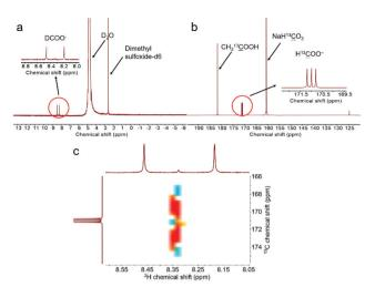
Fig. 5 D-qNMR (a), <sup>13</sup>C-qNMR (b) and COSY spectra (c) of the liquid sample after NaH13CO3 reaction with methanol in D2O (reaction conditions:  $0.1 \text{ mol L}^{-1} CH_3OH$ ,  $1 \text{ mol L}^{-1} NaH^{13}CO_3$ ,  $50\% D_2O$  filling, 50 mgPd<sub>0.5</sub>Cu<sub>0.5</sub>/C, 180 °C, and 16 h; dimethyl sulfoxide-D6 and CH<sub>3</sub><sup>13</sup>COOH were used as the internal standards to calculate the D-labelled and <sup>13</sup>C-labelled formate concentrations, respectively).
