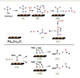
Fig. 7 Reaction scheme of HCO<sub>3</sub><sup>-</sup> reduction into formate with methanol in water on the Pd<sub>0.5</sub>Cu<sub>0.5</sub>/C catalyst.
