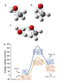
Fig. 4 Transition states (a)–(c) and energy profiles (d) for methanol dissociation into  $H_2$  with or without  $H_2O$  (a: methanol molecule; b: the transition state without  $H_2O$ ; c: the transition state with  $H_2O$ ; and d: the profile with  $H_2O$  as the promoter is depicted in orange, while the profile without  $H_2O$  is depicted in blue).
