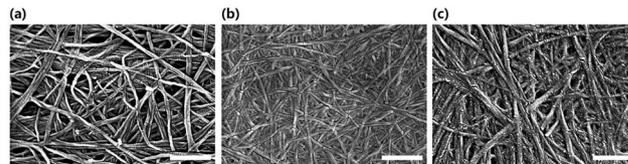
**Fig. 2** SEM images of (a) pure BC, (b) conventional TEMPO-oxidised CNF and (c) CNF obtained in one-pot over Siliacat TEMPO. Scale bar = 500 nm. [Reproduced from ref. 14, Creative Commons Attribution (CC BY) license].
