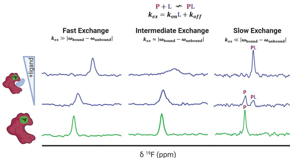
Fig. 8 Idealized spectra of protein-observed  $^{19}\text{F}$  NMR with ligands. Ligands in fast chemical exchange (left), intermediate exchange (middle), and slow exchange indicating the distinct states of free (P) and bound (PL) protein (right).
