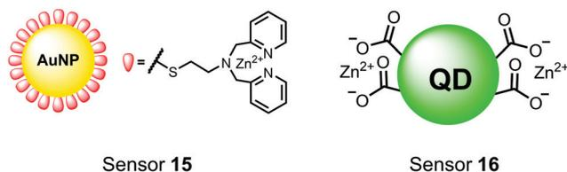
Fig. 6 Structures of inorganic nanoparticle sensors **15** and **16**.
