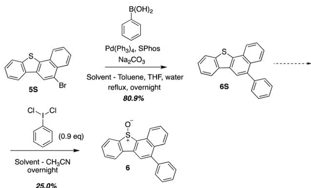
Scheme 3 Synthesis of **6** which represents the core structure of **2** and **3**.
