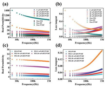
Frequency dependences of dielectric permittivity and loss tangent for (a and b) single layer and (c and d) bilayer composites.
