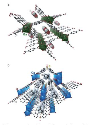
Fig. 3 Incommensurate metal-organic frameworks. Representations of (a) IM-19 ps and (b) Ca(sbd). Guest H<sub>2</sub>BDC molecules for IM-19 ps and guest n-pentane molecules for Ca(sbd) were added by the artist to illustrate a possible pore filling configuration.
