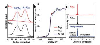
Fig. 5 (a) Au 4f XPS and (b) Au  $L_3$ -edge XANES profiles of  $Au_{21}$ (-SR) $_{12}$ (Ph $_2$ PCH $_2$ PPh $_2$ ) $_2$  and  $Au_{23}$ (SR) $_{16}$ . (c) The  $^1$ H NMR spectra of Auacetylide species.
