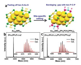
Fig. 3 (a) A schematic diagram of the site-specific editing of  $Au_{23}(SR)_{16}$  by resecting two RS-Au-SR motifs and bandaging the gaps with two  $Ph_2P-CH_2-PPh_2$  staples to obtain  $Au_{21}(SR)_{12}(Ph_2PCH_2PPh_2)_2$ . Color codes: yellow = Au; green = S; pink = P; blue = C. Carbon tails are omitted for clarity. SR = cyclohexanethiol. The ESI-MS spectra of (b)  $[Au_{23}(SC_6H_{11})_{16}]^-$  and (c)  $[Au_{21}(SC_6H_{11})_{12}(Ph_2PCH_2PPh_2)_2]^+$ .
