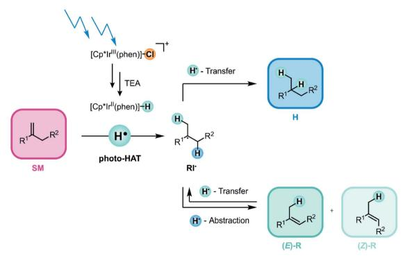
Fig. 2 Visible-light driven catalytic hydrogenation of electron-neutral olefins based on photo-triggered hydrogen atom transfer (photo-HAT) from an iridium( $\shortparallel$ ) hydride (Cp\* = pentamethylcyclopentadienyl; phen = 1,10-phenanthroline), see text for details.
