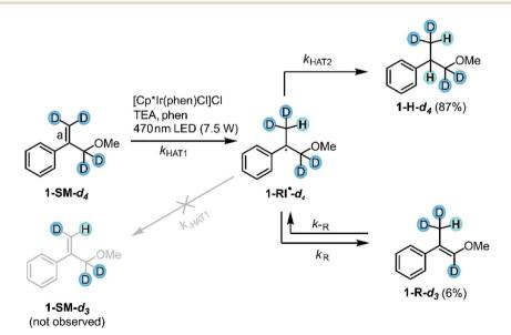
Fig. 9 Experiment with deuterated substrate 1-SM- $d_4$ : no proton incorporation into the terminal double bond (bond labeled "a") was observed, indicating that H-atom abstraction from 1-RI $^{-}$ - $d_4$  to afford 1-SM- $d_3$  is negligible (crossed gray leftward arrow labeled  $k_{-HAT1}$ ). For simplicity, only the (E)-isomer of the rearranged product 1-R- $d_3$  is shown.
