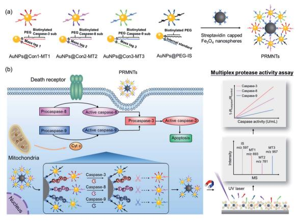
Scheme 1 Schematic design of the core-satellite PRMNTs for activity assay of intracellular caspases in apoptosis. (a) Preparation of the PRMNTs by coupling streptavidin capped magnetic Fe<sub>3</sub>O<sub>4</sub> nanospheres with a series of satellite AuNPs co-decorated with mass tags and biotinylated linkers. (b) The principle of quantifying the intracellular activity of cascaded caspases in apoptosis pathways by using the core-satellite PRMNTs.
