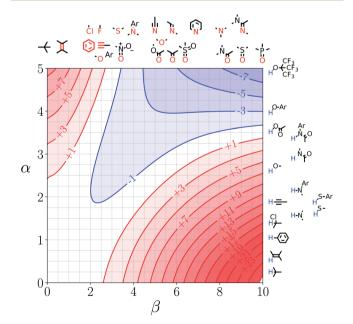
Fig. 7 FGIP for the interaction of two solutes in formic acid at 298 K ( $\Delta\Delta G_{\rm FGI}$  in kJ mol $^{-1}$ ). The solute–solute interactions in the blue region, and unfavourable in the red region.
