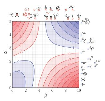
Fig. 4 FGIP for the interaction of two solutes in water at 298 K ( $\Delta\Delta G_{\rm FGI}$ in kJ  $mol^{-1}$ ). The solute-solute interactions are favourable in the blue region, and unfavourable in the red region.
