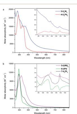
Fig. 7 UV-Vis absorption spectra of  $3-U_2Ni_2$  and  $4-U_2Pd_2$  (a),  $5-(UNi)_n$ , 6-UPd, and  $7-U_2Pt_3$  (b) measured in THF at rt. Inset: near infrared absorption spectra.
