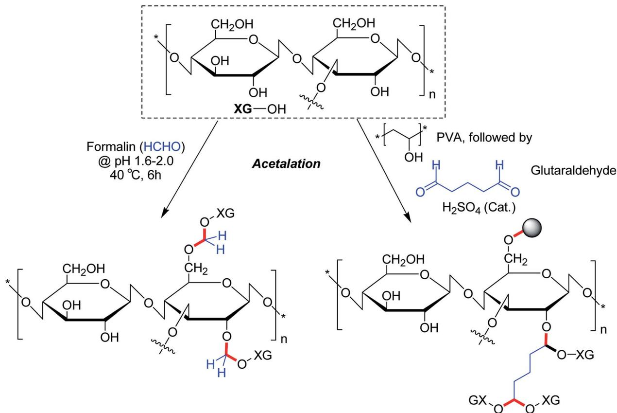
Fig. 15 Acetalation of XG using formaldehyde and glutaraldehyde.
