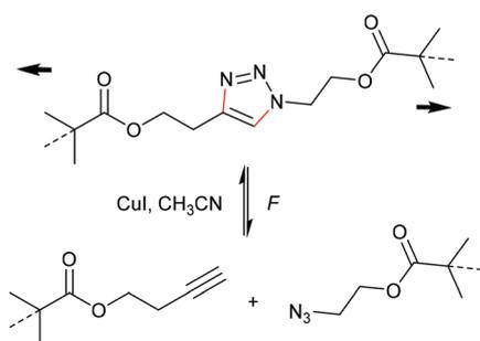
**Scheme 19** Supposed force-induced cycloelimination of the triazole mechanophore yielding azide and alkyne moieties.<sup>98,99</sup>
