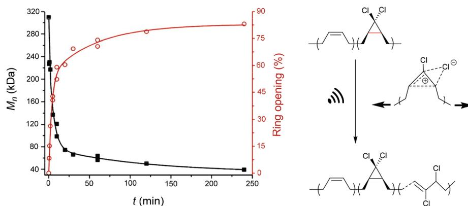
Fig. 4 Ultrasonication of gDCC-PB copolymer leads to ring-opened 2,3-dichloroalkenes (○) with simultaneously decreasing  $M_n$  (■). Adapted with permission from ref. 120. Copyright 2009 American Chemical Society.
