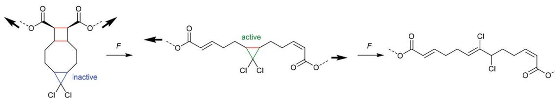
**Scheme 12** Copolymer of cyclobutane- and *gDCC*-based mechanophores to achieve a mechanical gating effect.<sup>55</sup>
