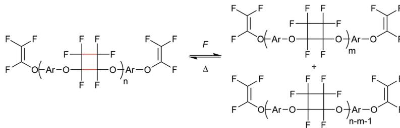
**Scheme 4** Structure of the PFCB mechanophores capable of thermal healing after mechanical damage.<sup>30</sup>
