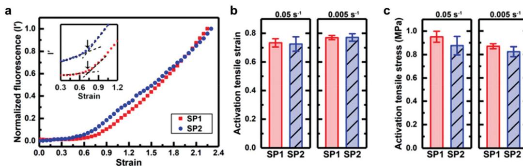
**Fig. 8** Activation behaviour of SP1 or SP2 incorporated in PDMS under tension: comparison of (a) the normalized fluorescence intensity as a function of strain at a strain rate of  $0.05\text{ s}^{-1}$ ; (b) the onset of activation strain; (c) the activation stress.<sup>219</sup> Reprinted with permission from ref. 219. Copyright 2018, American Chemical Society.
