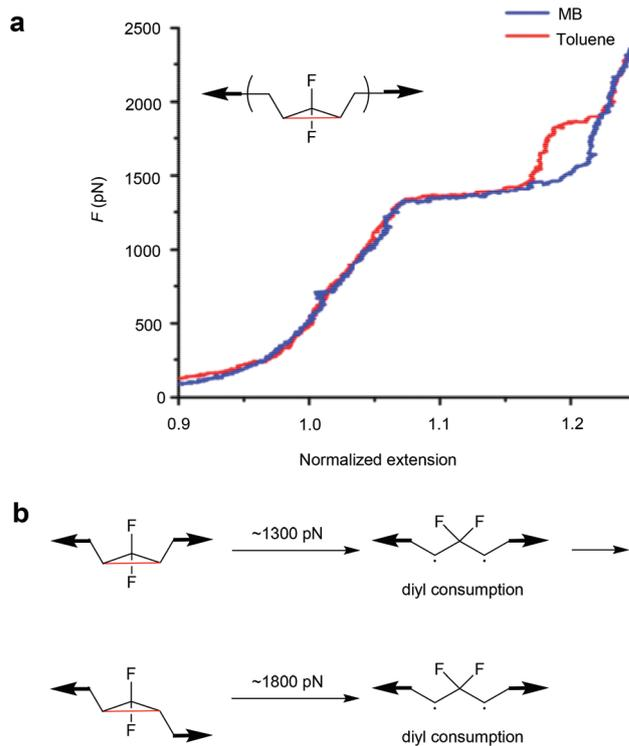
Fig. 6 (a) Representative SMFS force curves of *Z*-*g*DCC polymer obtained in MB (blue) and toluene (red). (b) The mechanistic scheme for *Z*-*g*DCC when the SMFS experiment is performed in toluene. Adapted with permission from ref. 137. Copyright 2016 American Chemical Society.
