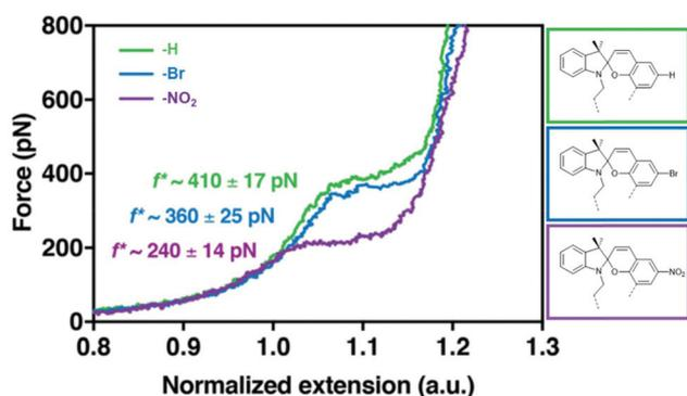
Fig. 10 SMFS curves for SP2 derivatives with *para*-H, -Br or -NO<sub>2</sub> and their transition force  $f^*$ .<sup>222</sup> Adapted with permission from ref. 222. Copyright 2018 American Chemical Society.
