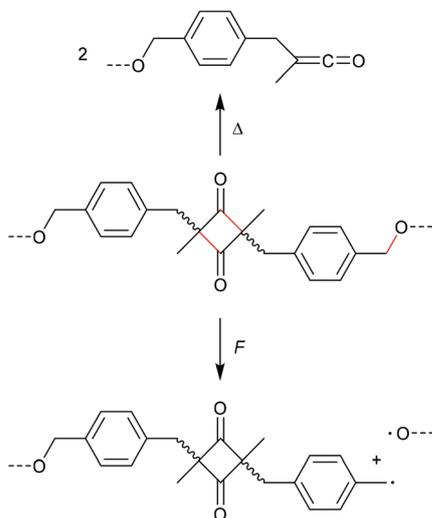
**Scheme 8** Application of heat or force to a ketene dimer bearing polymer substituents in 2,4-position.<sup>35</sup>
