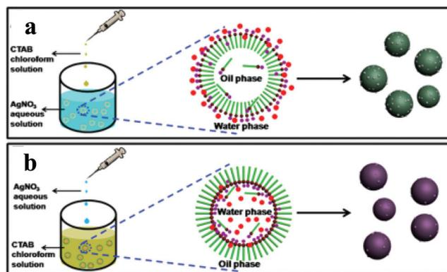
Fig. 9 Schematic explanation for the one-pot surfactant-assisted synthesis of Ag/AgBr-based nanostructures *via* an oil/water (a) and a water/oil (b) microemulsion system. Copyright 2012, American Chemical Society. Reprinted from ref. 84 with permission.
