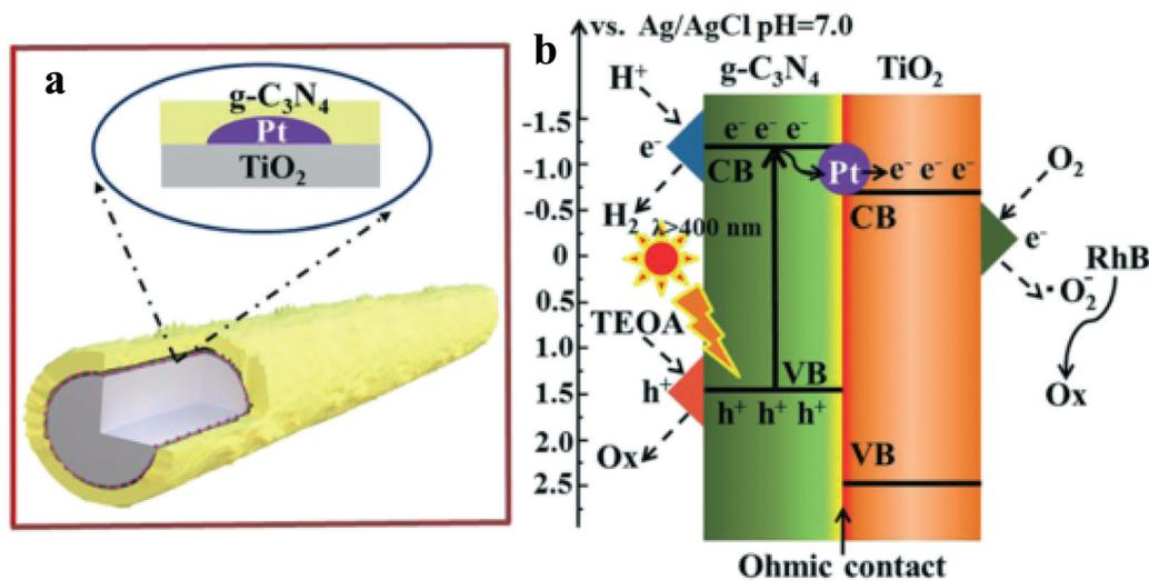
Fig. 6 Schematic structure (a) and the photogenerated electron–hole transfer pathways (b) inside the CN/Pt/TiO<sub>2</sub> composite under visible light irradiation. Copyright 2019, Royal Society of Chemistry. Reprinted from ref. 39 with permission.
