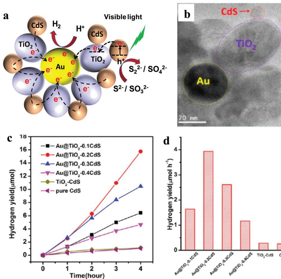
Fig. 5 (a) Schematic illustration of photocatalytic activity of the Au@TiO<sub>2</sub>-CdS nanocomposite, (b) TEM, (c) plots of the photocatalytic HER versus visible light irradiation time and (d) HER for pristine CdS, binary TiO<sub>2</sub>-CdS and various ternary nanocomposites. Fig. 4b–d: Copyright 2013, American Chemical Society. Reprinted from ref. 35 with permission.
