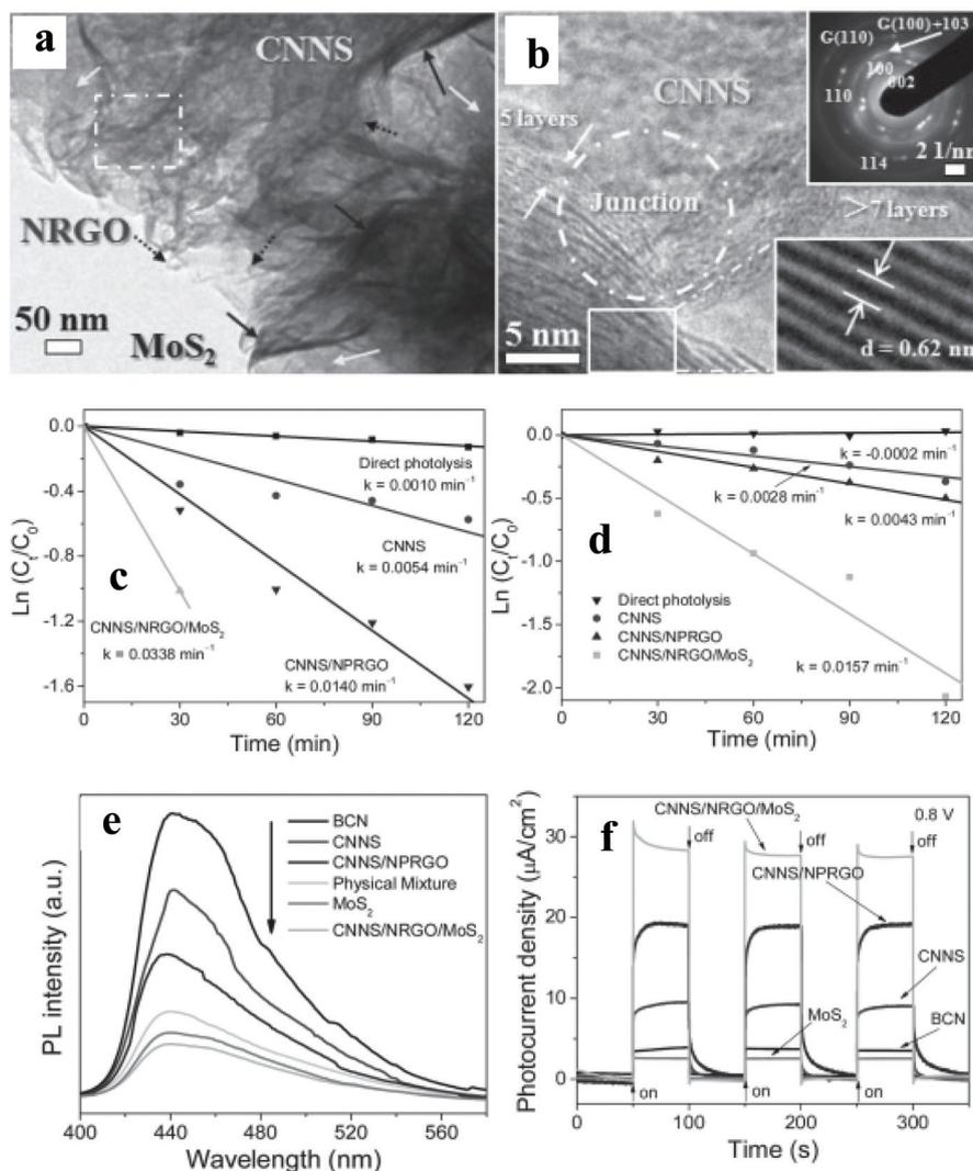
Fig. 7 (a and b) TEM images, SAED pattern, and HRTEM images of CNNS/NRGO/MoS<sub>2</sub> nanojunctions, (c and d)  $\ln(C_t/C_0)$  of MB and Cr(VI) versus time for different photoactive materials under simulated sunlight irradiation, (e) PL spectra and (f) transient photocurrent density versus Na<sub>2</sub>SO<sub>4</sub> electrolyte. Copyright 2013, Wiley Online Library. Reprinted from ref. 53 with permission.
