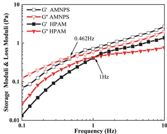
Fig. 7 Viscoelasticity of HPAM and MANPS.
