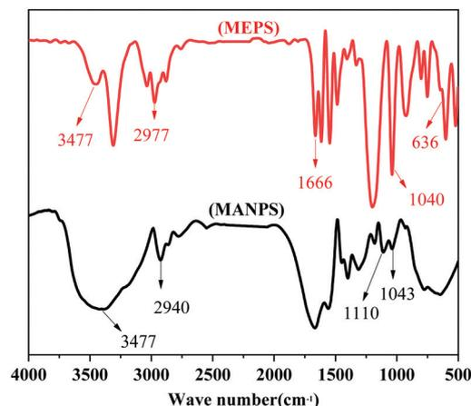
**Fig. 2** FT-IR spectra of MEPS and MANPS.
