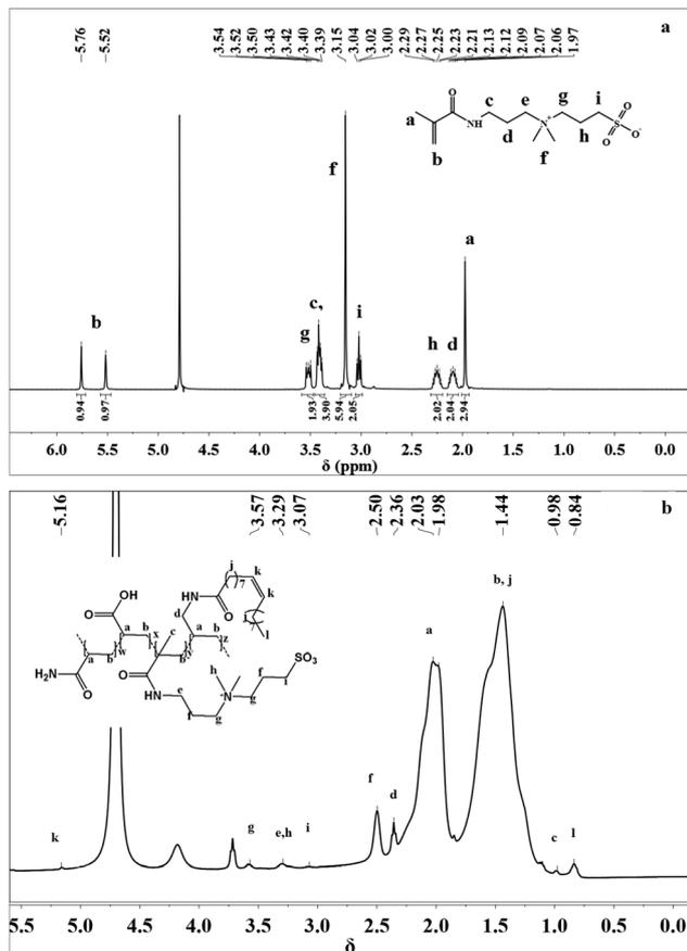
Fig. 3  $^1\text{H}$  NMR spectra: MEPS (a) and MANPS (b).
