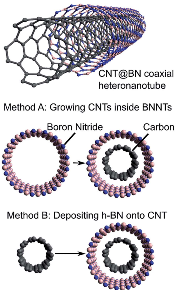
Fig. 1 Schematic depiction of CNT@BN coaxial heteronanotube and methods of synthesis by (A) growing CNTs inside BNNTs or (B) depositing h-BN onto CNT. Only SWCNT and single layer h-BN are depicted here for simplicity.
