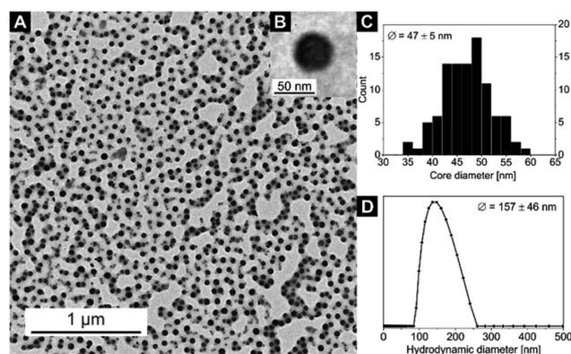
Fig. 2 (A) TEM image of sample **4**, the cores of the micelles with the embedded  $[\text{Zn}(\text{OAc})_2(\text{bipy})]_n$  CP nanoparticles appear black, (B) an inset with a zoom on a single nanoparticle, (C) core size distribution  $D_{\text{core}}$  (from TEM) and (D) hydrodynamic diameter distribution  $D_h$  (from DLS) of the nanocomposite sample **4** (for DLS autocorrelation function see Fig. S6†).
