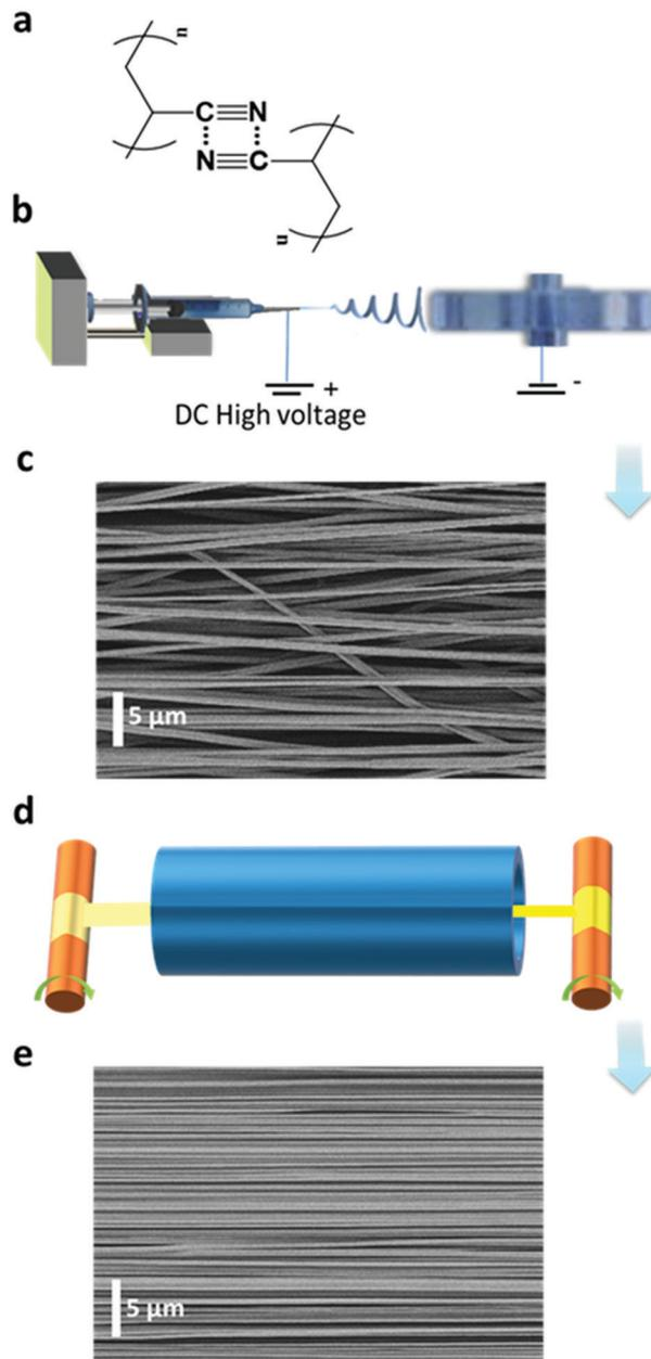
**Fig. 1** Fabrication process and microstructure of ENRs. (a) Chemical structure of PAN with dipole-dipole attraction interactions. (b) Electrospinning setup. (c) A SEM image of the PAN as-spun ENRs. (d) Roll-to-roll heat-stretching setup. (e) A SEM image of the PAN ENRs after the heat-stretching process with a stretch ratio of six.
