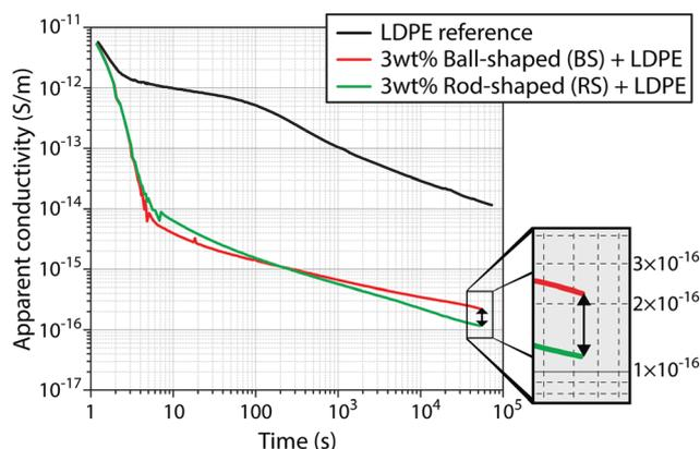
Fig. 2 Apparent conductivity of composites containing 3 wt% ball- or rod-shaped particles and of pristine LDPE at 30 kV mm<sup>-1</sup> at 60 °C. Several measurements up to 2 days were made independently on separately prepared samples, see Fig. S2 (ESI†).
