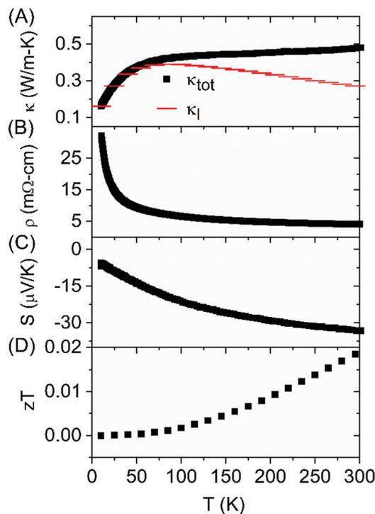
Fig. 5 Total thermal conductivity ( $\kappa_{\text{tot}}$ ) and lattice thermal conductivity ( $\kappa_l$ ) (A), resistivity (B), Seebeck coefficient (C), and  $zT$  (D) measured on a  $\text{FeAs}_{1.50}\text{Se}_{0.50}$  single crystal.
