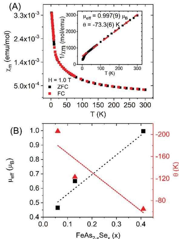
Fig. 4 (A)  $\chi_m$  vs.  $T$  for  $\text{FeAs}_{1.50}\text{Se}_{0.50}$  single crystals (FC is shown in red, ZFC is shown in black). The inlay shows  $1/\chi_m$  vs.  $T$  with the Curie-Weiss fit from 100 K to 300 K. (B) Calculated values of  $\mu_{\text{eff}}$  and  $\theta$  (K) vs. Se fraction ( $x = 0.06$  and  $0.13$  are from literature).<sup>10</sup>
