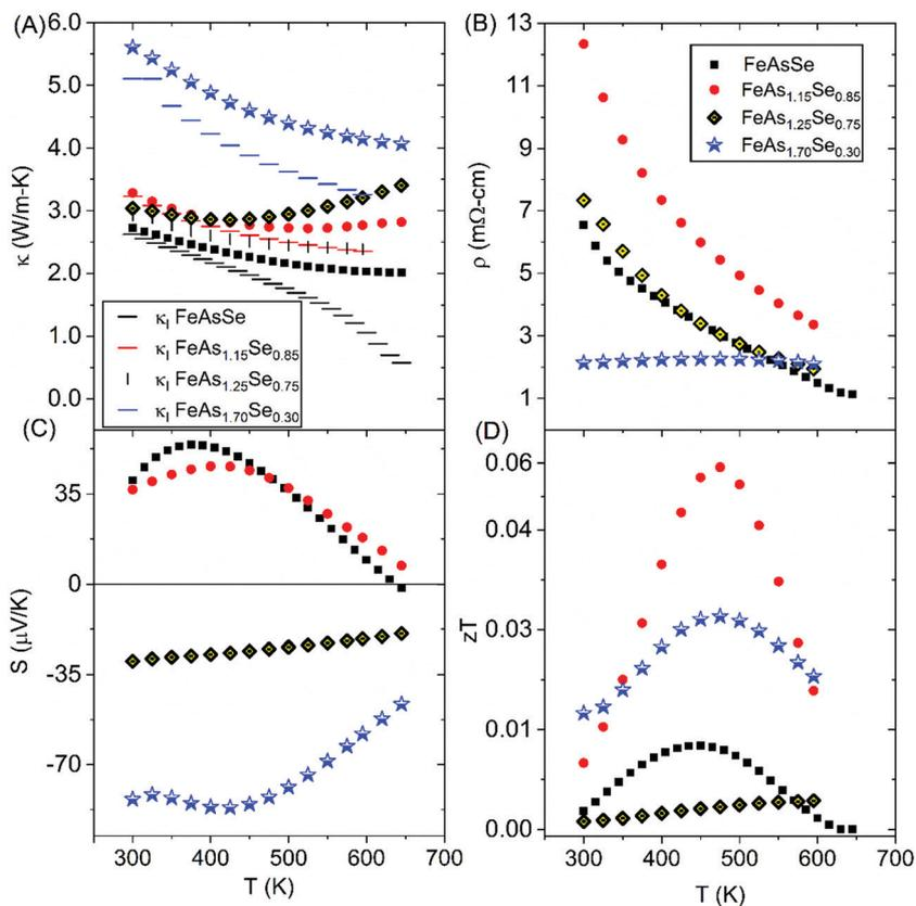
Fig. 6 Total thermal conductivity ( $\kappa_{\text{tot}}$ ) given as symbols and lattice thermal conductivity ( $\kappa_l$ ) provided as dashes (A), resistivity (B), Seebeck coefficient (C), and  $zT$  (D) measured on sintered polycrystalline pellets of  $\text{FeAs}_{2-x}\text{Se}_x$  ( $x = 0.3, 0.75, 0.85, 1.0$ ).
