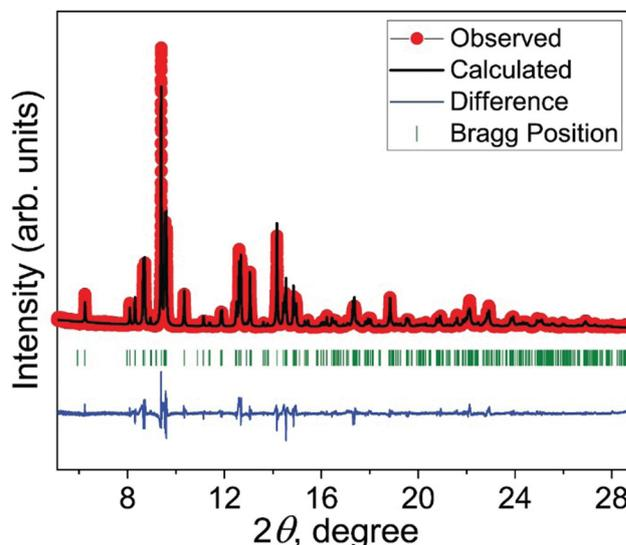
Fig. 2 Rietveld refinement of synchrotron PXRD pattern of  $\text{FeAsSe}$  (arsenopyrite structure type, space group  $P2_1/c$ ). Color code: red dots = observed pattern, black line = calculated pattern, green bar = Bragg position, blue line = difference between observed and calculated patterns.
