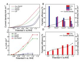
Fig. 3 (A) LSV curves of various electrodes with a scan rate of 50 mV $^{-1}$ ; (B) the FE of  $C_2H_4$  at -1.2 V (vs. RHE) over various electrodes; (C) partial current density of  $C_2H_4$  over various electrodes at different applied potentials; (D) the FE and current density of  $C_2H_4$  over Cu-Pd/CP at different applied potentials in  $CO_2$ -saturated 0.1 M KCl solution.
