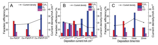
Fig. 4 The FE of  $C_2H_4$  over Cu-Pd bimetallic catalysts (A) using different electrodeposition methods; (B) under different current densities; (C) obtained at various deposition times.
