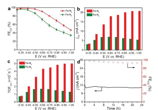
Fig. 3  $CO_2$  electroreduction catalytic performance of Fe-N<sub>5</sub> and Fe-N<sub>6</sub>. (a) Faradaic efficiency of CO at different potentials. (b)  $j_{CO}$  in 1.0 M KOH electrolyte. (c)  $TOF_{CO}$  at various applied potentials. (d) 24 h stability test of Fe-N<sub>5</sub> at -0.4 V vs. RHE and the corresponding  $FE_{CO}$ .
