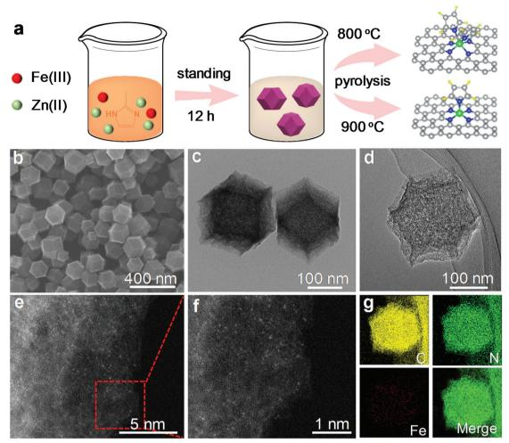
Fig. 1 (a) Schematic of the formation process of Fe $-N_5$  and Fe $-N_5$ . (b) SEM, (c) TEM, and (d) HAADF-STEM images of Fe $-N_5$ . (e) and (f) Magnified HAADF-STEM images of Fe $-N_5$  demonstrate the atomic dispersion of Fe atoms. (g) EDS elemental mapping reveals the homogeneous distribution of Fe. N. and C in Fe $-N_5$ .
