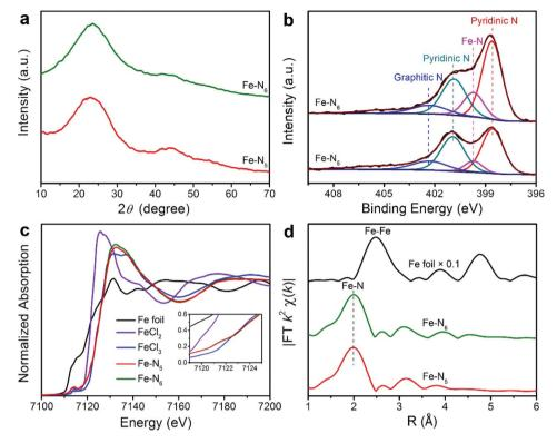
Fig. 2 (a) XRD patterns of Fe-N<sub>5</sub> and Fe-N<sub>6</sub>. (b) High-resolution N 1s XPS spectra of Fe-N<sub>5</sub> and Fe-N<sub>6</sub>. (c) Fe K-edge XANES spectra of Fe-N<sub>5</sub>, Fe-N<sub>6</sub> and Fe foil/FeCl<sub>2</sub>/FeCl<sub>3</sub> reference materials. (d) Fe K-edge  $k^2$ -weighted FT-EXAFS spectra of Fe-N<sub>5</sub>, Fe-N<sub>6</sub>, and Fe foil.
