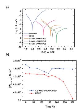
Fig. 6 (a) PDP curves for bare steel, pure CPUD and composite coatings in 3.5 wt% NaCl solution; and (b) plots of  $|Z|_{0.01~Hz}$  against the immersion time for pure CPUD and the 1.0 wt% cPANI/CPUD composite coating.
