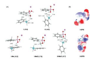
**Fig. 3** DFT-calculated interaction modes. (A) Optimized complex structures of sodium aryl borates (**3j**, **3k**, and **3o**) with phenylsilane at the M06-2X-D3/6-311G(d, p) level of theory in solvent. Values in parenthesis denote the binding energies (in kcal mol $^{-1}$ ) calculated at the DSD-PBEP86/def2-TZVPP level in solvent. Bond lengths are in Å. (B) Electrostatic potential map for the catalyst–silane interaction.
