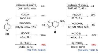
Fig. 5 Comparison results of borate-catalysis approach with non-catalytic methods.
