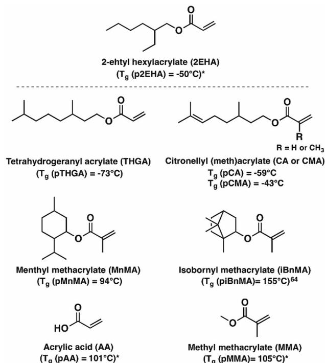
Fig. 1 The structure of 2-ethyl hexyl acrylate, the four terpenoid-based (meth)acrylate monomers combined with acrylic acid and methyl methacrylate used in the PSA formulations. \*The values for  $T_g$  were adopted from Sigma-Aldrich.
