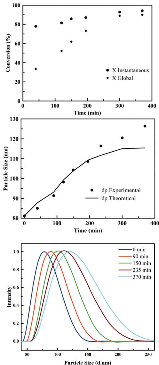
Fig. 2 The conversion as a function of time (top), the evolution of the particle size as a function of time (middle) and the corresponding DLS traces (bottom) of **PSA2** during feeding in the seeded semi-batch emulsion polymerization.
