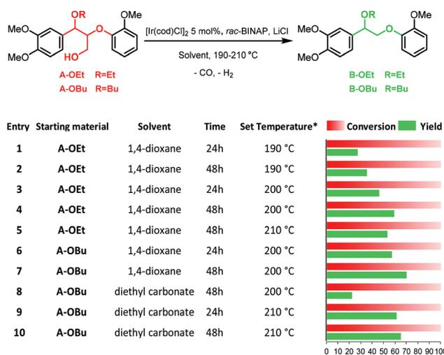
**Fig. 6** Catalytic dehydrogenative decarbonylation A-OEt or A-OBu to B-OEt or B-OBu. Reaction conditions: 15 mg substrate,  $[\text{Ir}(\text{cod})\text{Cl}]_2$  5 mol%, 4 : 2 : 1 LiCl : *rac*-BINAP :  $[\text{Ir}(\text{cod})\text{Cl}]_2$ , as catalyst; 190–210 °C in 1 mL solvent. Yield and conversion were determined by GC-FID using *n*-decane as an external standard; \*Set temperature of the heating block; the measured corresponding inside temperature is shown in Table S1.†
