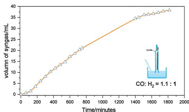
**Fig. 5** Syngas formation over time using 4-hydroxy-3-methoxybenzenepropanol (BP2) as a model compound. Reaction conditions: 1 mmol substrate,  $[\text{Ir}(\text{cod})\text{Cl}]_2$  2.5 mol%, *rac*-BINAP 5 mol%, LiCl 10 mol%, 190 °C (setting temperature of the oil bath) in 2 mL solvent. Yield and conversion were determined by GC-FID using *n*-ocatadecane as external standard.
