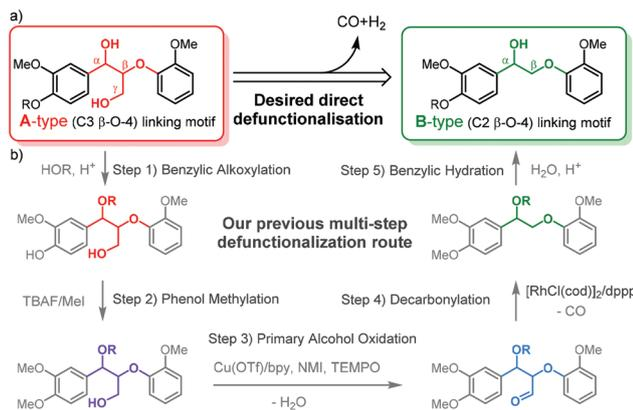
**Fig. 1** (a) The two types of  $\beta$ -O-4 linkage motifs commonly represented in model compounds used in the chemical methodology development for lignin valorisation and (b) multistep defunctionalisation of alcohol incorporated organosolv lignin via methylation, oxidation and decarbonylation demonstrated in our previous work.<sup>31</sup>
