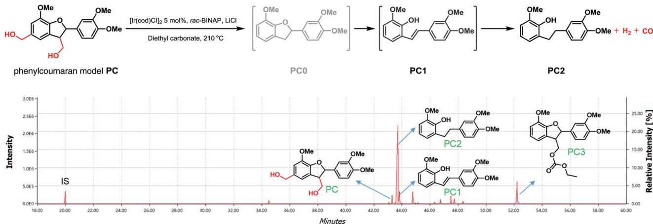
Fig. 7 Dehydrogenative decarbonylation of the phenylcoumaran model compound (PC). Reaction conditions: 10 mg substrate,  $[\text{Ir}(\text{cod})\text{Cl}]_2$  5 mol%, 4 : 2 : 1 LiCl : *rac*-BINAP :  $[\text{Ir}(\text{cod})\text{Cl}]_2$ , heating block set at 210 °C in 1 mL solvent.
